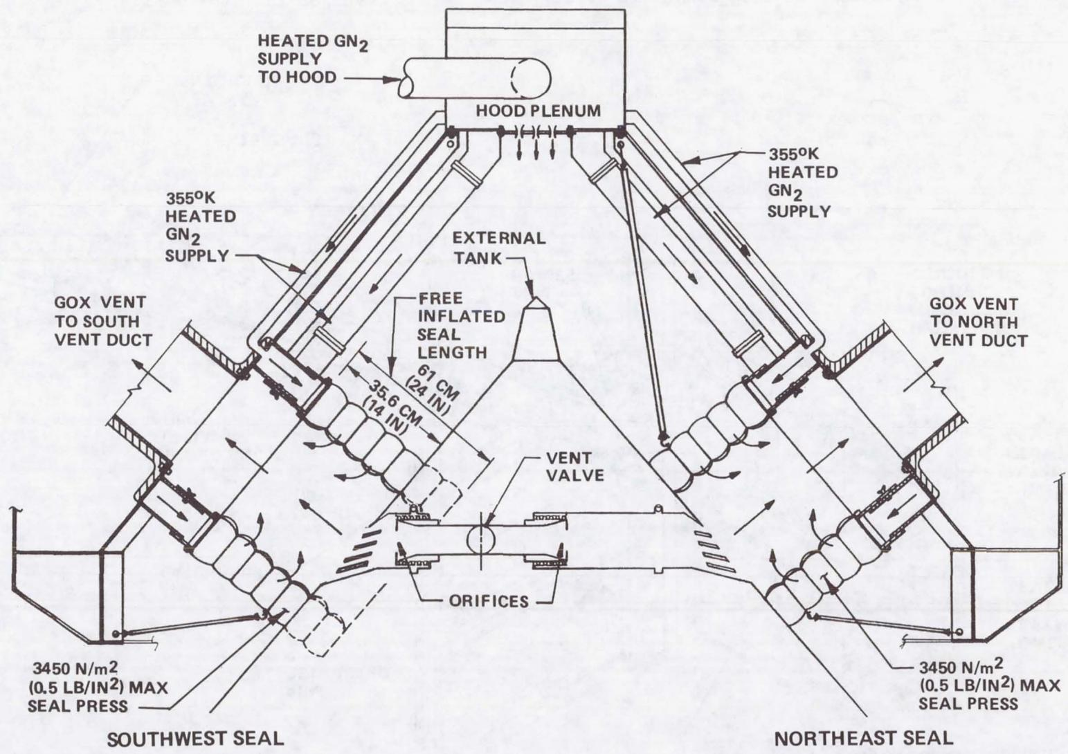
Figure 2. Vent Hood Cutaway Showing Vent Seals and Interface With ET
